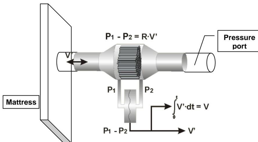
In this experiment, air was pumped in and out through the measuring apparatus as in the previous experiment. That is, with a calibrating syringe (50cc) at a rate of 30/min. Flow rates and pressure were continuously measured. Resistance to flow is defined as the ratio of the two:
