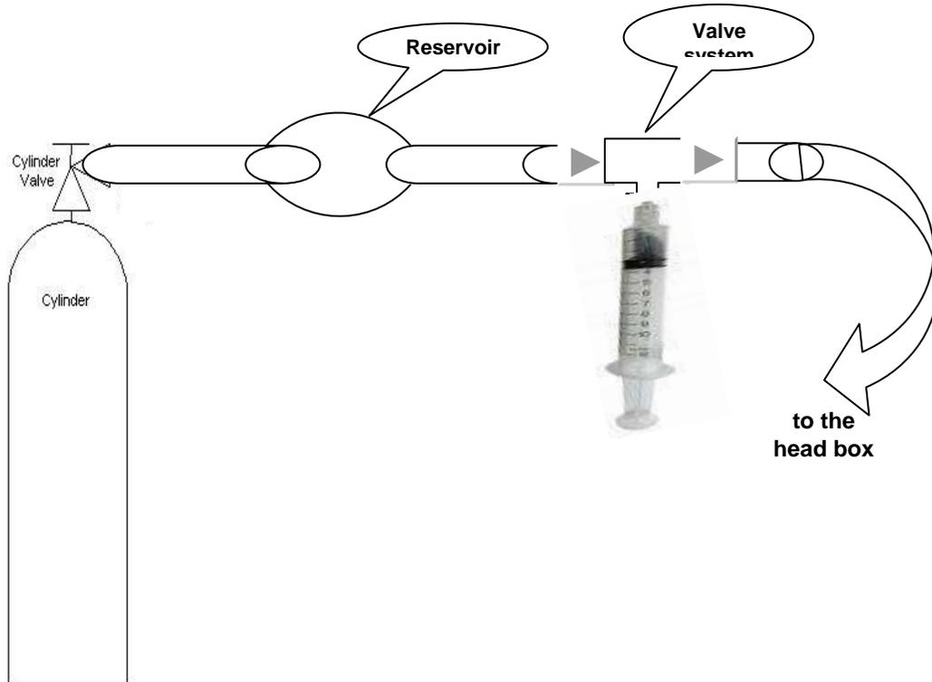
The valve system was constructed of two one-way valves arranged in a way to allow unidirectional flow, left-to-right in this case (Fig.2). Air always came in from the reservoir (on the left) which was continuously filled with a gas mixture of known CO<sub>2</sub> concentration (4.8% was chosen because it is similar to expired CO<sub>2</sub> levels in human beings). Air out (to the right) was directed into the headbox.
